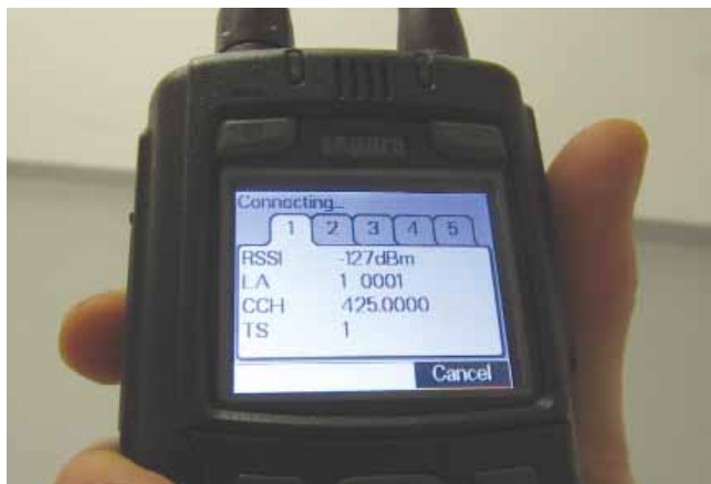
Top left: Repeater installed into one underground tunnel in the Yas Marina Circuit area. Top right: Field strength with the repeater off. Left: An uplink antenna receiving the base station's signal and delivering it to the repeater.
